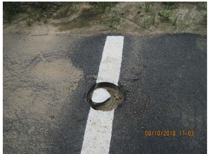
Picture – 23: Photo of 7" dia. core hole in pavement.
